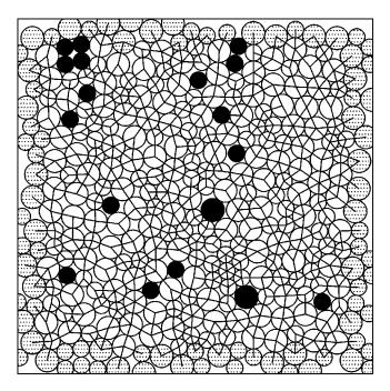
FIG. 6. Collectively jammed bidisperse disk packing. The algorithm to test for collective jamming in ideal packings was applied to this equimolar bidisperse disk packing of 250 disks ( $\varphi$ =0.846) in order to identify a jammed subpacking of 232 disks, leaving 18 rattlers (colored black), which are not essential for jamming. The dotted disks represent periodic images. Note that the density would be significantly lowered if the rattling particles were removed.
