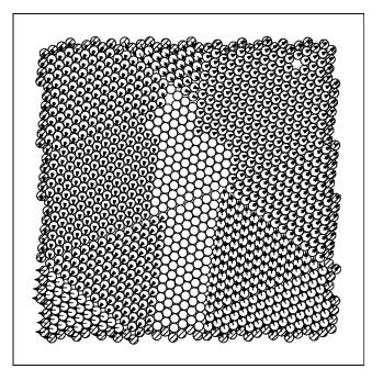
FIG. 8. Collectively jammed disk packing. A dense ( $\varphi = 0.89$ ) random packing of 1000 disks that is collectively jammed but not strictly jammed, and a representative unjamming motion. One can see the grains gliding over each grain boundary due to the shear, bringing this packing closer to a triangular lattice
