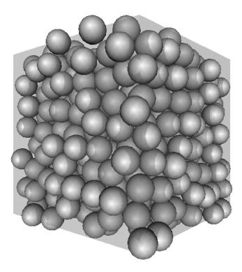
FIG. 5. Virtually strictly jammed sphere packing. This random packing of 500 spheres with density  $\varphi$ =0.64 was produced using the (original) Lubachevsky–Stillinger algorithm and it is collectively jammed and practically strictly jammed. The (cubical) unit cell is also shown.
