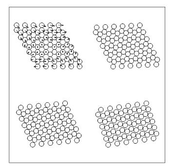
FIG. 3. Shearing the honeycomb lattice. The honeycomb lattice is not strictly (or collectively) jammed, and an example of a lattice deformation, replicated on several unit cells to illustrate the shear character of the strain  $\varepsilon = (\Delta \Lambda) \Lambda^{-1}$ . Note that only three (original) spheres are involved in the actual calculation of this unjamming motion, the rest are image spheres.
