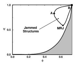
FIG. 1. A highly schematic plot of the jammed subspace in the density-disorder plane.
